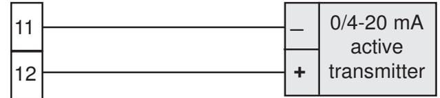
Fig. 100/4-20 mA input wiring for active transmitter
