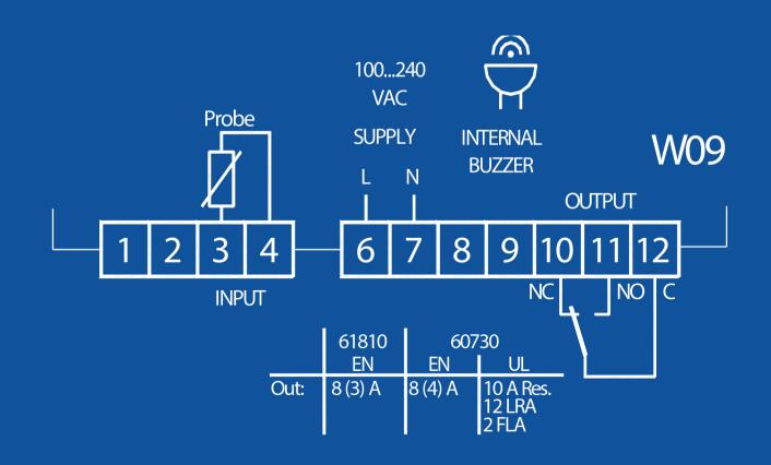
1 - MODEL W09 - WALL MOUNTED TEMPERATURE CONTROLLER **2 - POWER SUPPLY** H = 100... 240 VAC/DC L = 24 VAC/DC**3 - OUTPUT** R = Out Replay SPDT 8A-AC1 HOW TO ORDER 4 - BUZZER B = Buzzer included - = None **USE THIS GUIDE TO FIND THE PART NUMBER OF** THE PRODUCT YOU WANT
