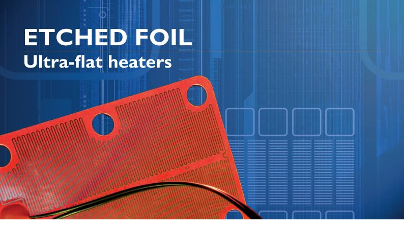
Flexible ultra-flat heaters are produced using etchedfoil technology on a silk-screened circuit, which is then coupled with insulating materials such as silicone, polyester, polyimide (kapton®), teflon and mica, depending on operating temperatures.
