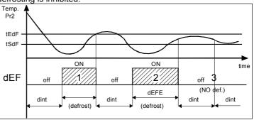
Examples: defrosting 1 ends due to reaching of temperature "tEdF", defrosting 2 ends at the end of the "dEFE" time as the temperature "tEdF" is not reached, defrosting 3 does not take place as the temperature is higher than "tSdF".
