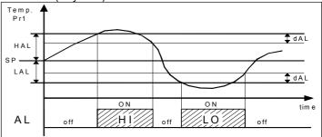
The maximum and minimum temperature alarms can be disabled by setting the relative parameters "HAL" and "LAL" = OFF. At the same time as the signalling of the configured alarm (buzzer
