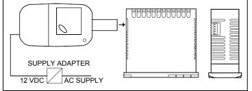
To transfer the configuration of an instrument into the device **(UP-LOAD)** it is necessary to proceed in the following way:
