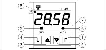
${\bf 1}$  -  ${\bf Key}\ {\bf P}$  : Used for the set point setting and to program the functioning parameters
