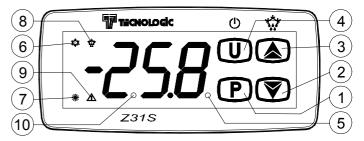
**1 - Key P**: Used for setting the Set point (press and release) and for programming the function parameters (hold pressed for 5 sec.) In programming mode is used to enter in parameters edit mode and confirm the values.
