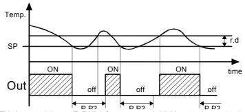
Third control (par. "P.P3") foresees an inhibition to the activation of the output "Out" by a time delay that starts when the output was turning on last time (delay between switching-on).
