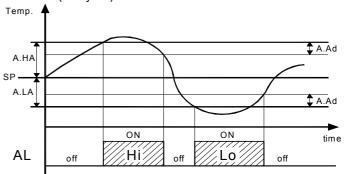
The maximum and minimum temperature alarms can be disabled by setting the relative parameters "A.HA" and "A.LA" = oF.
