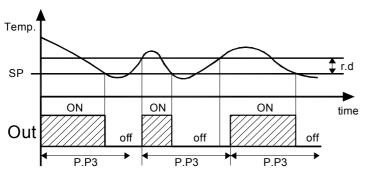
During the output inhibition the led OUT (Cool o Heat) blinking. It is also possible to prevent activation of the output after the instrument is turned on, for the time set in the parameter "**P.od**". During the power on delay phase, the display shows the indication **od**, alternating with the normal visualisation.
