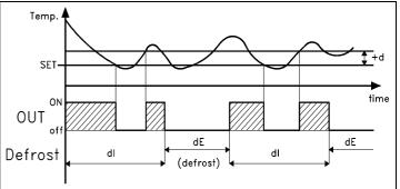
The occurring defrost cycle is signalized by the label "dF" appearing on the display.
