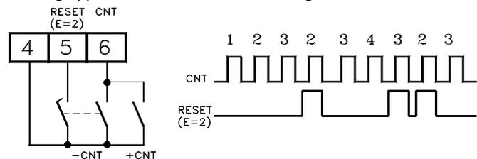
With this UP/DOWN counting applications the counting cannot assume negative values and therefore reached the value 0 (counting UP) or the set value (counting DOWN) others pulses can't be acquired.
