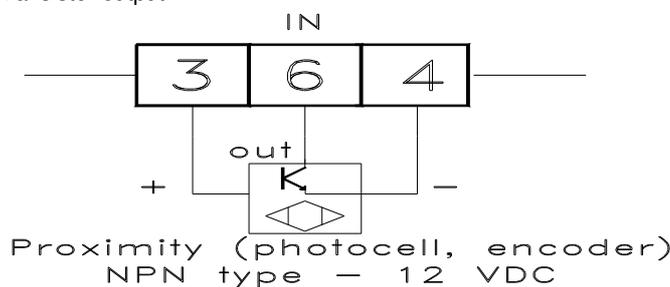
In order to the counting frequency is advisable to program the filter software of the par. "H" that it allows to select the maximum counting frequency and to avoid
