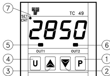
**1 - Key P** : Used for the set point setting and to program the functioning parameters
