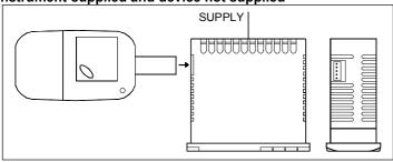
Instrument supplied from the device
