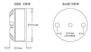
Fixing holes 2 x  $\emptyset$ 5.5 mm, Centre hole  $\emptyset$ 4.5 mm
