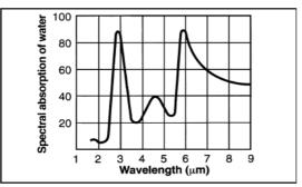
This diagram shows that water absorbs long wave infrared very well. Absorption maxima are approx. 3 and 6 µm
