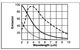
Emission spectrum of black body radiators. Dotted Line: 2100°C (as for visible radiators); Solid Line: 1100°C (as for quartz radiators); Dashed Line: 510°C for ceram ic radiators, best range 3 to 10  $\mu m$ .
