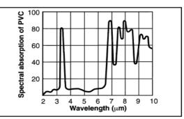
This is the spectral absorption of PVC. The main absorption range lies between 7 and 10  $\mu m$ . The curves for other plastics exhibit a similar character.
