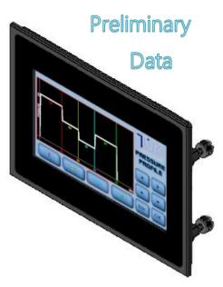
The resistive touch panel provides a cost effective one touch solution capable of accepting stylus, bare or gloved finger. The firmware can adjust sample rate, de-bounce, auto-repeat and acceptance area depending on required action. The bezel frame is symmetrical allowing 90 and 180 degree rotation with control by single software orientation command.
