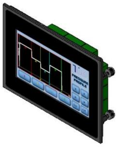
The resistive touch panel provides a cost effective one touch solution capable of accepting stylus, bare or gloved finger. The firmware can adjust sample rate, de-bounce, auto-repeat and acceptance area depending on required action. The bezel frame is symmetrical allowing 90 and 180 degree rotation with single software orientation command.
