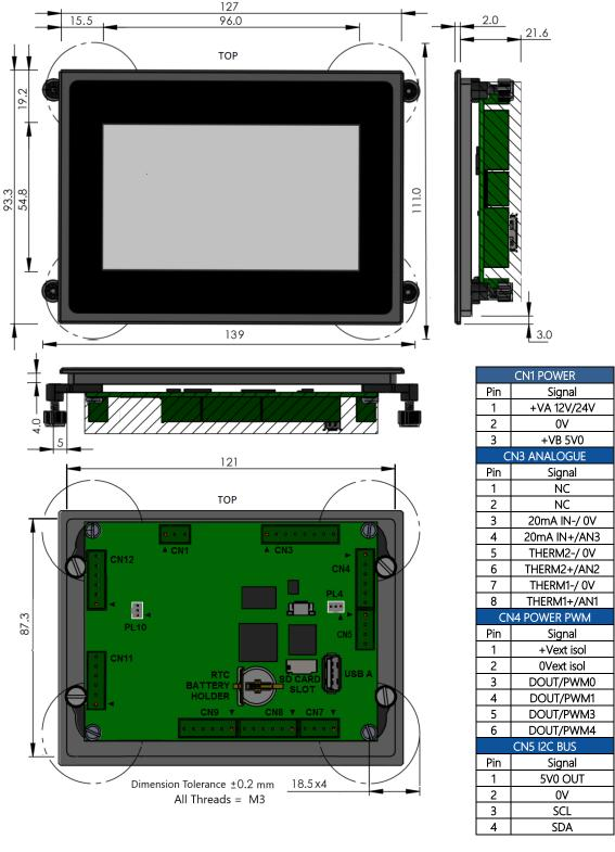
The +VB is a 5V output when +VA 12V/24V is applied.
