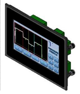
The resistive touch panel provides a cost effective one touch solution capable of accepting stylus, bare or gloved finger. The firmware can adjust sample rate, de-bounce, auto-repeat and acceptance area depending on required action. The bezel frame is symmetrical allowing 90 and 180 degree rotation with control by single software orientation command.
