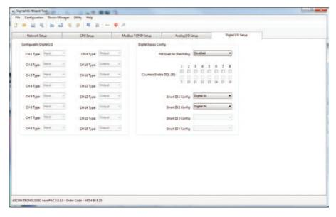
Note: The channels enabled in the "Configurable Digital I/O" part are automatically configured by the Wizard accordingly to the number of I/Os selected during the project creation. Note that the 16 digital I/O can freely be set only when the "16 Configurable Digital Channels + 2 Pulse Count" selection has been made.
