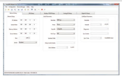
This page allows to configure the communication ports parameters.
