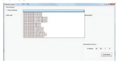
The new configuration screen is a very important page, as helps the user in determining the Hardware configuration of the CPU. It can be used online or offline (in the case the CPU is momentarily not connected to the PC).
