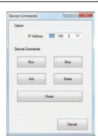
If needed, the selection of the "Erase PLC program" command will delete the PLC program from the media selected location: the overall time needed to perform the operation depends by the project size. Please wait until the "Persistency setup menu" screen reappears as confirmation for complete PLC program erasing.
